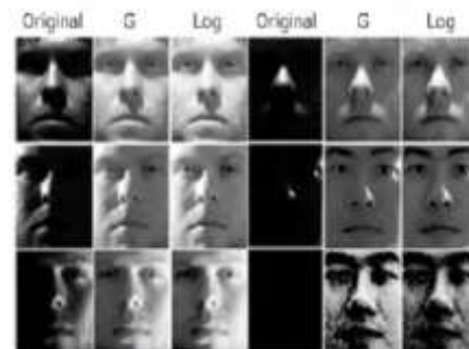
Fig.2. The results of gamma correction (G) and intensity logarithm (Log) applied on original images
